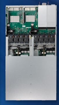
Alternatively, the dual PCI-E 3.0 x16 slots can support dual NVMeoF add-on-cards to enable additional deployment scenarios.
